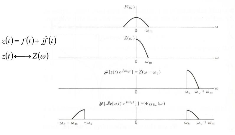
$$\phi_{\text{SSB+}}(t) = \text{Re}\left\{z(t) e^{j\omega_c t}\right\} = f(t)\cos(\omega_c t) - \hat{f}(t)\sin(\omega_c t)$$
