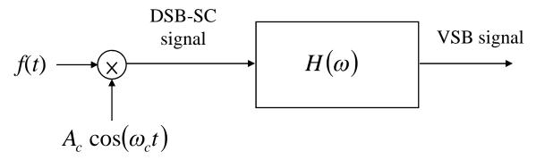
To determine the frequency-response characteristics of the filter, let us consider the demodulation for VSB signal.
