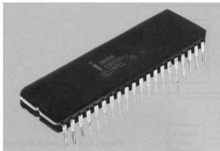
**Figure 1-5** Intel Corporation's 8086 Microprocessor.
