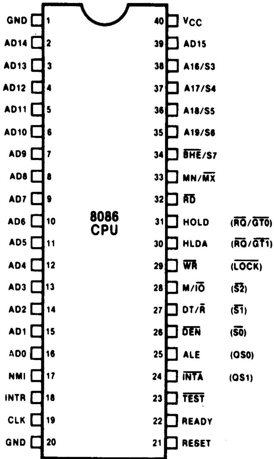
Figure 8-1 Pin layout of the 8086 Microprocessor.
