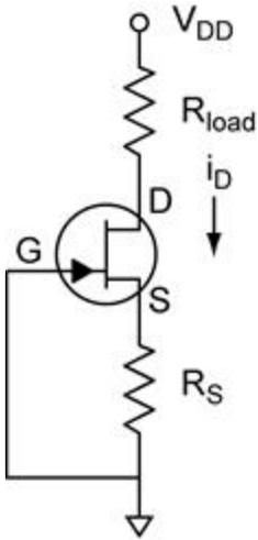
**Source Follower.** The simple source follower is shown below. The improved version is shown at the right. The lower JFET forms a current source. The result is that  $V_{GS}$  is held constant, removing the defects of the simple circuit.
