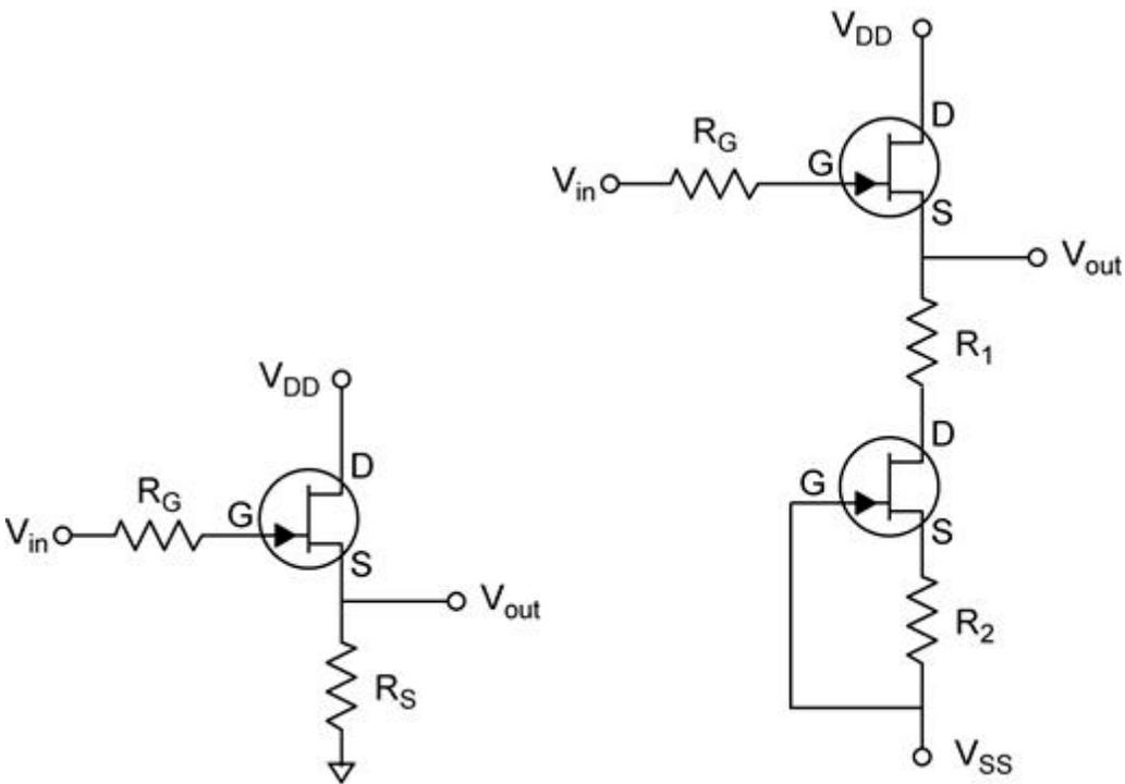
**Voltage-Controlled Resistor.**  $V_{GS}$  must be between zero and  $V_{GS,off}$ .
