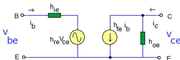
The hybrid model is suitable for small signals at mid band and describes the action of the transistor. Two equations can be derived from the diagram, one for input voltage  $v_{be}$  and one for the output  $i_c$ :
