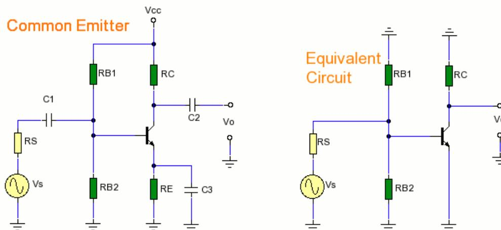
At ac the reactance of coupling capacitors C1 and C2 is so low that they are virtual short circuits, as does the bypass capacitor C3. The power supply (which will have filter
