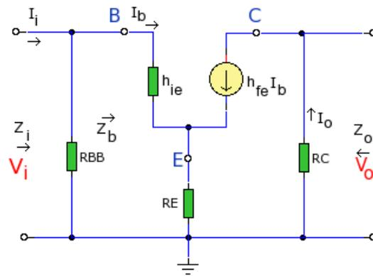
The current divider rule can be used for  $I_b$ :
