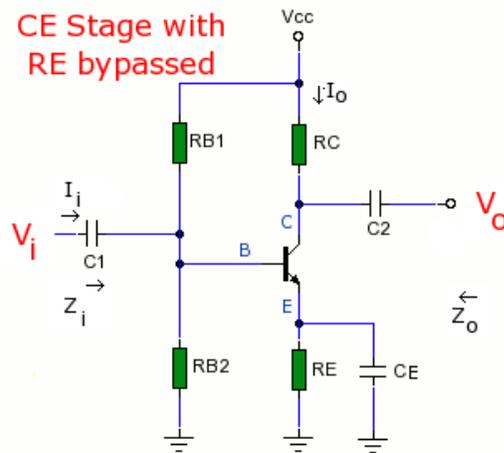
The small signal parameter  $h_{re}V_{ce}$  is often too small to be considered so the input resistance is just  $h_{ie}$ . Often the output resistance  $h_{oe}$  is often large compared with the collector resistor  $R_C$  and its effects can be ignored. The h-parameter equivalent model is now simplified and drawn below:
