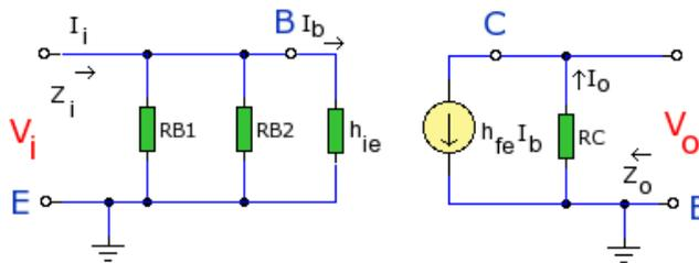
The current divider rule can be used for  $I_b$ :
