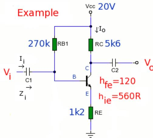
The hybrid parameters must be known to use the hybrid model, either from the datasheet or measured. In the above circuit,  $Z_i$ ,  $Z_o$ ,  $A_v$ , and  $A_i$  will now be calculated. Note that this CE stage uses a single bias resistor  $R_{B1}$  which is the value  $R_{BB}$ .
