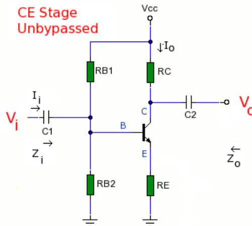
As in the previous example,  $R_{B1}$  and  $R_{B2}$  are in parallel, the bias resistors are replaced by resistance  $R_{BB}$ , but as  $R_E$  is now unbypassed this resistor appears in series with the emitter terminal. The hybrid small signal model is shown below, once again effects of small signal parameters  $h_{re}V_{ce}$  and  $h_{oe}$  have been omitted.
