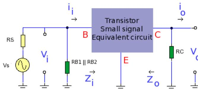
The blue rectangle now represents the small signal ac equivalent circuit and can now start work on the hybrid equivalent circuit.
