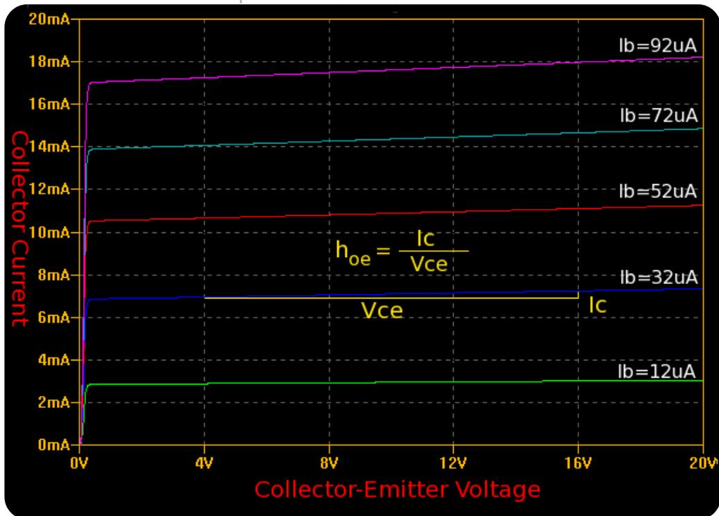
In addition, because the base currents are also known, then two small signal parameters,  $h_{fe}$  and  $h_{oe}$  can be determined straight from the graph. The almost flat portion of the curves, shows that the transistor behaves as a constant current generator. However, in saturation the steepness of the curves (between 0 and 0.4 Vce) show a sharp drop in  $h_{fe}$ . This is an important fact to consider, if using the transistor as a switch.
